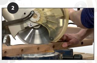
2. Transfer the same measurements to the other pre-drilled rail, set your saw to the pencil mark and trim both pre-drilled rails to the inside of the pencil mark on each end to allow for the width of the rail hanger bracket.
