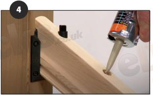
4. With the high-quality pink grip adhesive (sold separately), fill each pre-drilled hole about half way full. Then insert the angle adapters into the pre-drilled holes.
