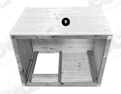
To fix the floor in place, we finally recommend screwing through the front and rear panels (A) and (B) using 3 x 75mm Green Coated Screws (FIX 2) on each, directly into the 2 x 2 timber that acts as the floor supports running underneath the kennel.
